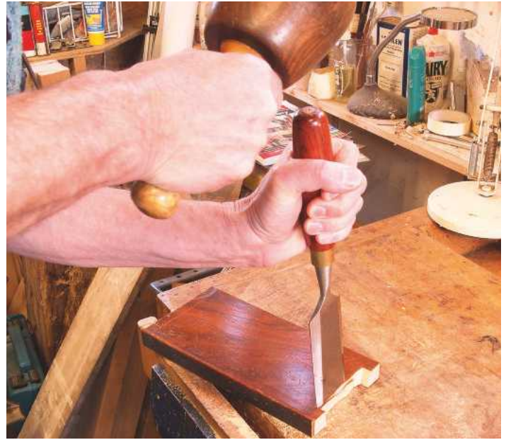
▲ Pic.11 Cleaning up pin board
